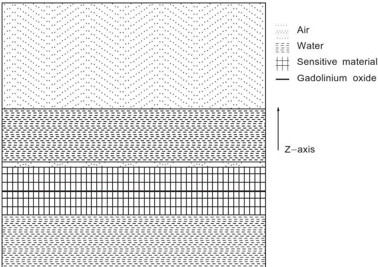
Dosimeter simulated as composed of various layers of alanine or ammonium tartrate and gadolinium
