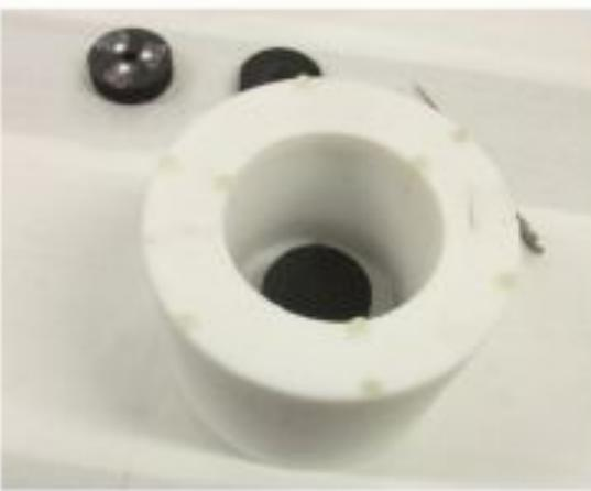
Shield for thermal neutrons composed of lithium carbonate enriched to 95% with  $^{6}\text{Li}$
