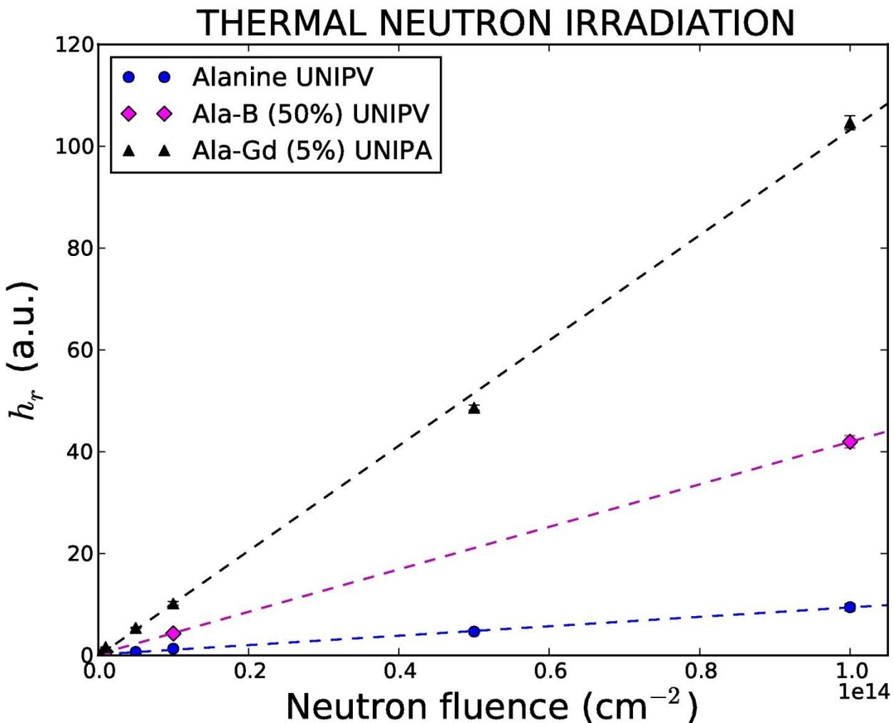
Gadolinium addition (5%) increases neutron sensitivity than Boron addition (50%)
