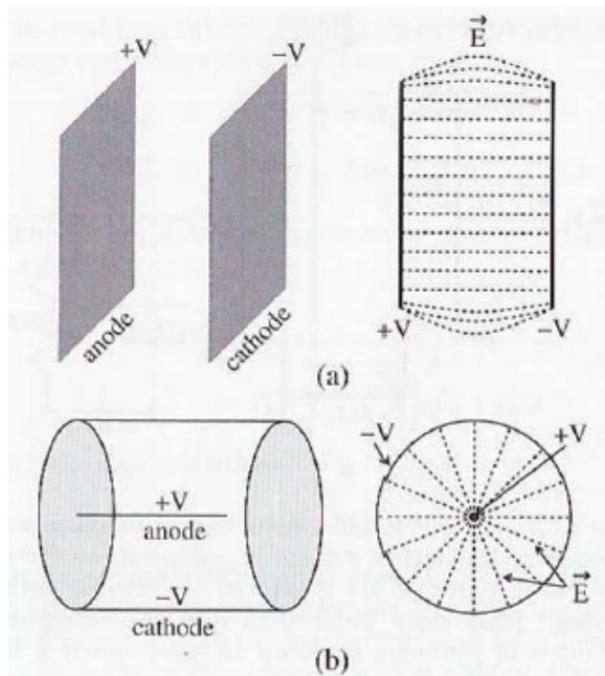
Figure 3.4.2: (a) Parallel plate ion chamber and a two dimensional view of electric field inside its active volume. The curved electric field at the sides may induce nonlinearity in the response. (b) Cylindrical ion chamber and a two dimensional view of radial electric field in its active volume. The increased flux of electric lines of force near the positively charged anode wire greatly enhances the electron collection efficiency.
