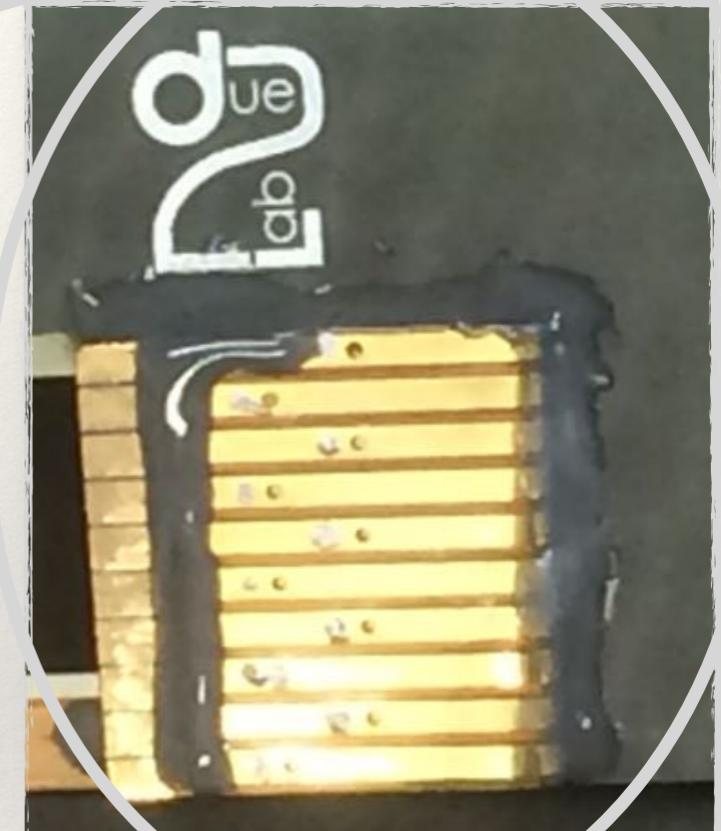
20 anode strips of pitch 1 mm
