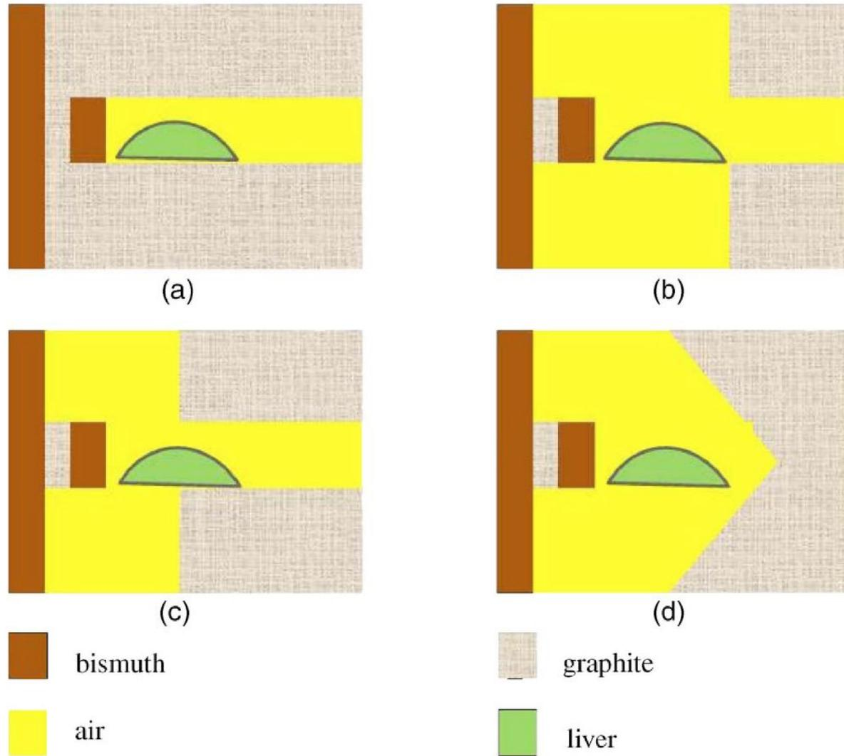
The different configurations tested were: a) the existing configuration used in patient treatment; b) larger open configuration; c) smaller open configuration; and d) closed conical-shaped channel configuration.
