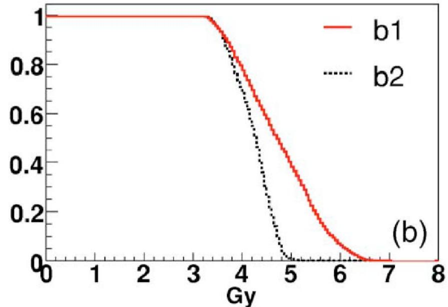
Differential DVH and integral DVH for graphite configuration in the actual facility and for the configuration b) with LiF absorber
