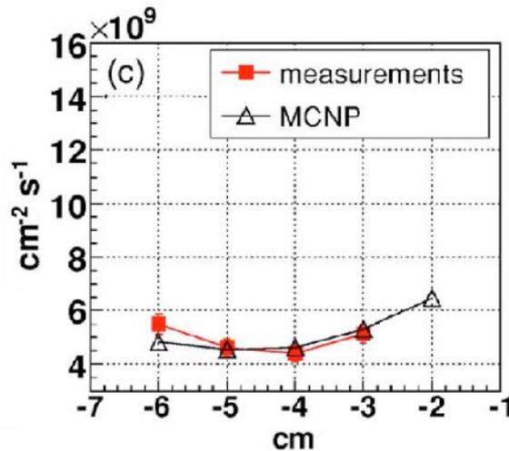
Thermal neutron flux distribution in the phantom filled with the hepatic-equivalent solution: along the  $x$ ,  $y$  and  $z$  axes
