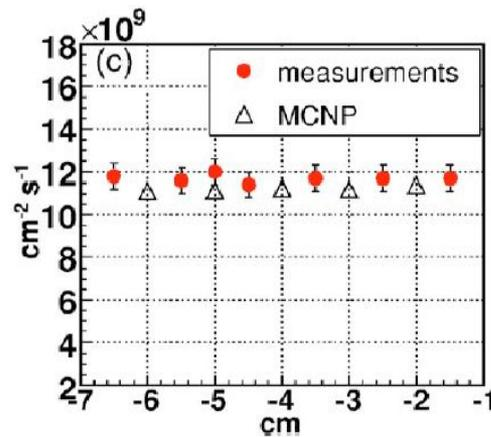
Thermal neutron flux distribution in the phantom filled with air along the  $x$ ,  $y$  and  $z$  axes
