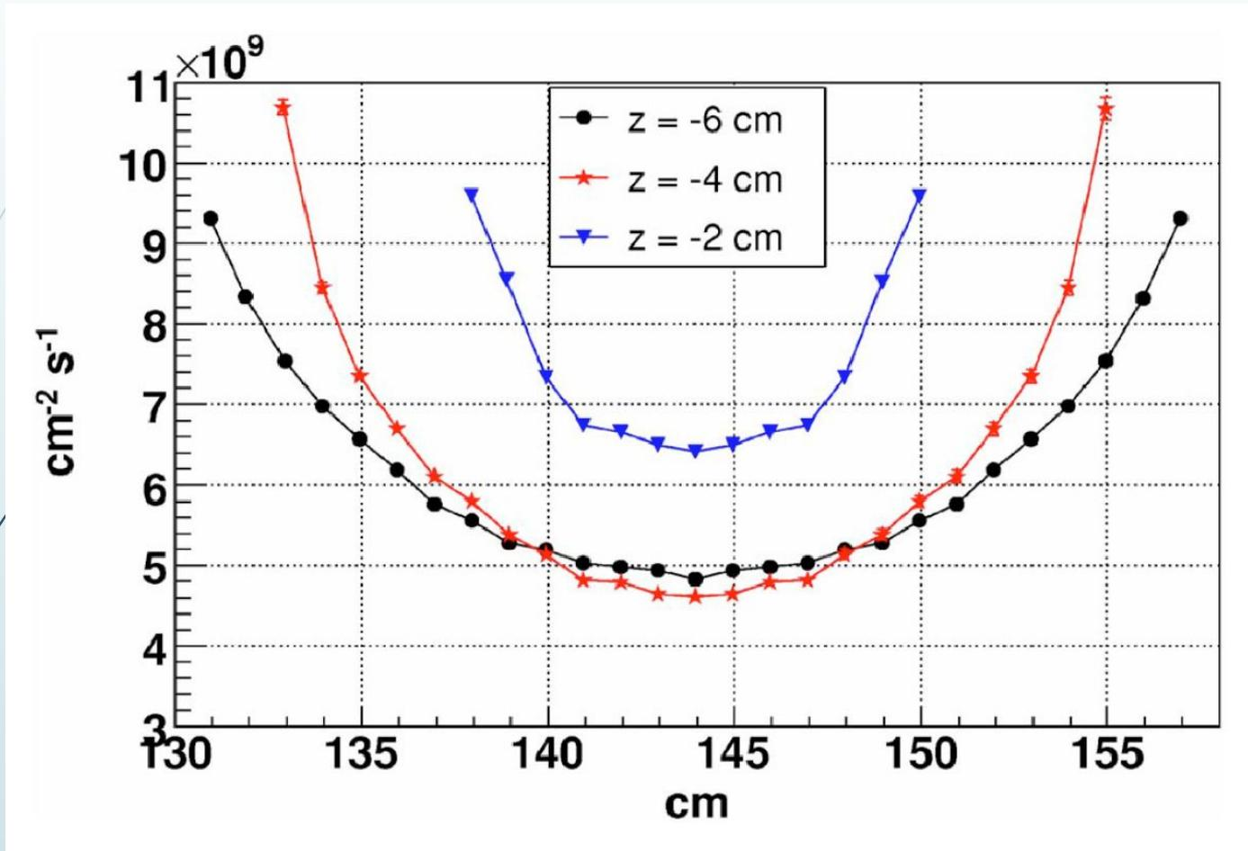
Calculated thermal neutron flux distribution along the longitudinal  $x$  axis after rotation of 180° at different positions along the  $z$  axis;
